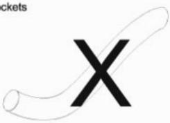
Note: Air in circuitry lines create noise and inhibit performance of Pulse Flow valve.
